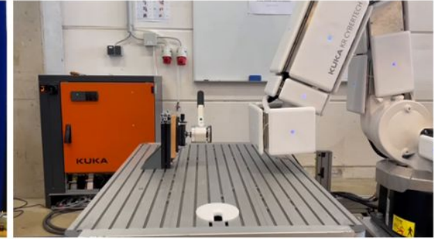
(c) KUKA Cybertech with AIRSKIN module pad (quasi-static contact).
